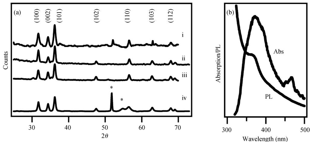
Fig. 1. (a) XRD patterns of ZnO (i) electrodeposited from  $\text{ZnCl}_2$  and (ii) electrodeposited from  $\text{Zn}(\text{NO}_3)_2$  solutions, (iii) electro-spun ZnO from  $\text{Zn}(\text{Ac})_2$  solution and (iv) ZnO-PS nanocomposite. The asterisk (\*) indicates XRD peaks of silicon. XRD patterns are shifted along the y-axis for clarity. (b) Absorption and photoluminescence spectra of electro-spun ZnO fibers.
