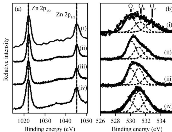
Fig. 4. (Colour online) XPS spectra of (a) Zn2p core levels and (b) O1s core level with Gaussian fits (dotted lines) for  $\text{O}_a$ ,  $\text{O}_b$  and  $\text{O}_c$ . Labels i, ii, iii and iv represent the same as Fig. 1(a). Spectra are shifted along the Y-axis for clarity.
