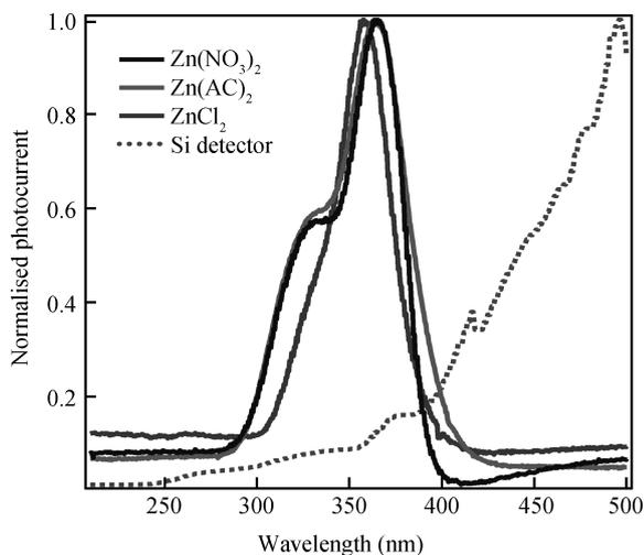
Fig. 3. Wavelength dependent photocurrent response of ZnO electro deposited thin films obtained from  $\text{Zn}(\text{NO}_3)_2$ ,  $\text{Zn}(\text{Ac})_2$  and  $\text{ZnCl}_2$  solutions. The bias voltage is set at 0 V. The spectral photocurrent response of the commercial Si detector is also included for comparison.
