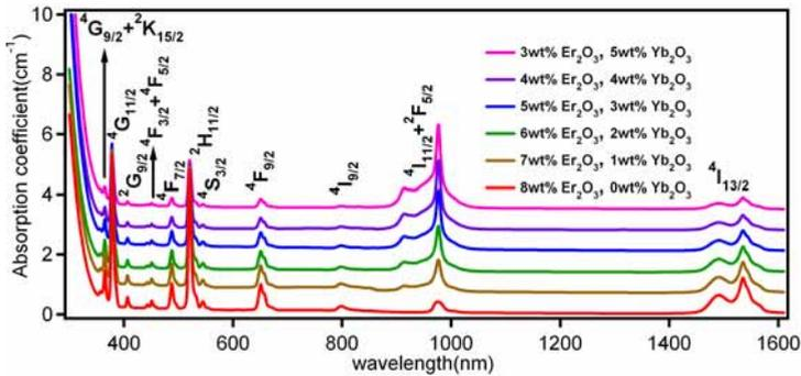
Fig. 3. Typical absorption spectra of Er<sup>3+</sup>/Yb<sup>3+</sup> co-doped phosphate (NAP) glasses.
