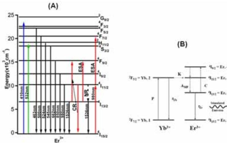
Fig. 2. (A) Partial electronic energy levels and various absorption and emission transitions of Er<sup>3+</sup> ions and (B) energy transfer between Er<sup>3+</sup> and Yb<sup>3+</sup> ions.
