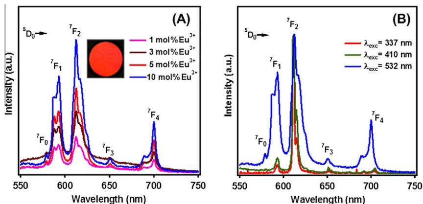
**Figure 2.** Room temperature emission spectra of (A)  $x$  mol% ( $x = 1, 3, 5, 10$ )  $\text{Eu}^{3+}$  doped in  $\text{KLaF}_4$  nanophosphor ( $\lambda_{\text{exc}} = 532$  nm) and (B) 10 mol%  $\text{Eu}^{3+}$ -doped  $\text{KLaF}_4$  nanophosphor with different excitation wavelengths.
