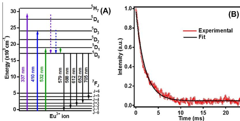
**Figure 3.** (A) Schematic excitation and emission transition energy level diagram of  $\text{Eu}^{3+}$  ion. (B) Representative emission decay curve for 612 nm ( ${}^5D_0 \rightarrow {}^7F_2$  of  $\text{Eu}^{3+}$ ) emission of 10 mol%  $\text{Eu}^{3+}$ -doped  $\text{KLaF}_4$  nanophosphor ( $\lambda_{\text{exe}} = 532$  nm).
