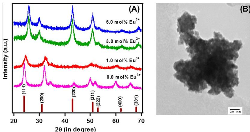
**Figure 1.** Room temperature (A) X-ray diffraction pattern of  $x$  mol% ( $x = 0, 1, 3, 5$ )  $\text{Eu}^{3+}$ -doped  $\text{KLaF}_4$  nanophosphor. The XRD patterns were indexed according to the JCPDS data No. 75–2020. (B) TEM image of 5 mol%  $\text{Eu}^{3+}$ -doped  $\text{KLaF}_4$  nanophosphor.
