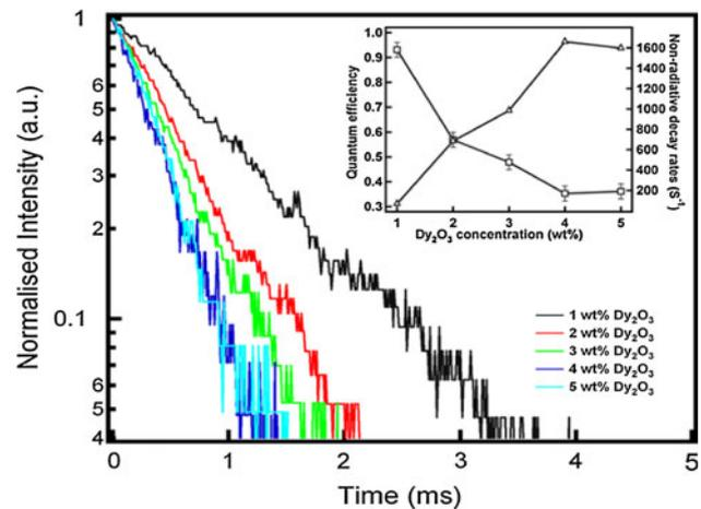
**Fig. 3** Decay curves of <sup>4</sup>F<sub>9/2</sub> level monitored at <sup>4</sup>F<sub>9/2</sub> → <sup>6</sup>H<sub>13/2</sub> transition in various wt% Dy<sub>2</sub>O<sub>3</sub>-doped NAP glasses. Inset shows the variation of quantum efficiency and non-radiative decay rate of <sup>4</sup>F<sub>9/2</sub> level with Dy<sub>2</sub>O<sub>3</sub> concentration
