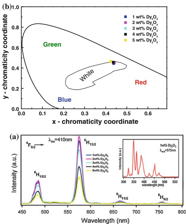
**Fig. 2** a Emission spectra of various wt%  $\text{Dy}_2\text{O}_3$ -doped NAP glasses. The inset shows the excitation spectra of 575 nm emission of 1 wt%  $\text{Dy}_2\text{O}_3$ -doped NAP glass. b CIE coordinate diagram of various  $\text{Dy}^{3+}$ -doped NAP glasses by 410 nm excitation
