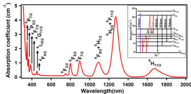
**Fig. 1** Absorption spectrum of 2 wt% Dy<sub>2</sub>O<sub>3</sub>-doped NAP glasses. Inset shows the partial energy level diagram of Dy<sup>3+</sup> ions in NAP glass
