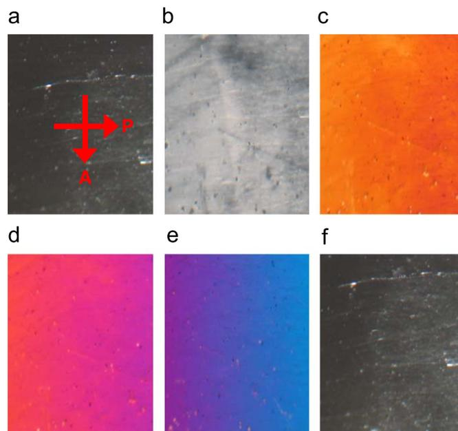
**Fig. 2.** (Colour online) Optical micrograph (magnification of  $50\times$ ) of homeotropically aligned nematic liquid crystal cell (silane treatment with gentle rubbing) at room temperature at (a) 0V, (b) 2.5V, (c) 4.5V, (d) 6V, (e) 10V, and (f) 0V after 10V.
