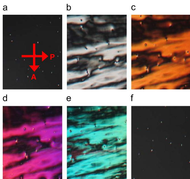
**Fig. 1.** (Colour online) Optical micrograph (magnification of  $50\times$ ) of homeotropically aligned nematic liquid crystal cell (without any surface treatment) at room temperature at (a) 0V, (b) 3V, (c) 4V, (d) 4.5V, (e) 10V, and (f) 0V after 10V.
