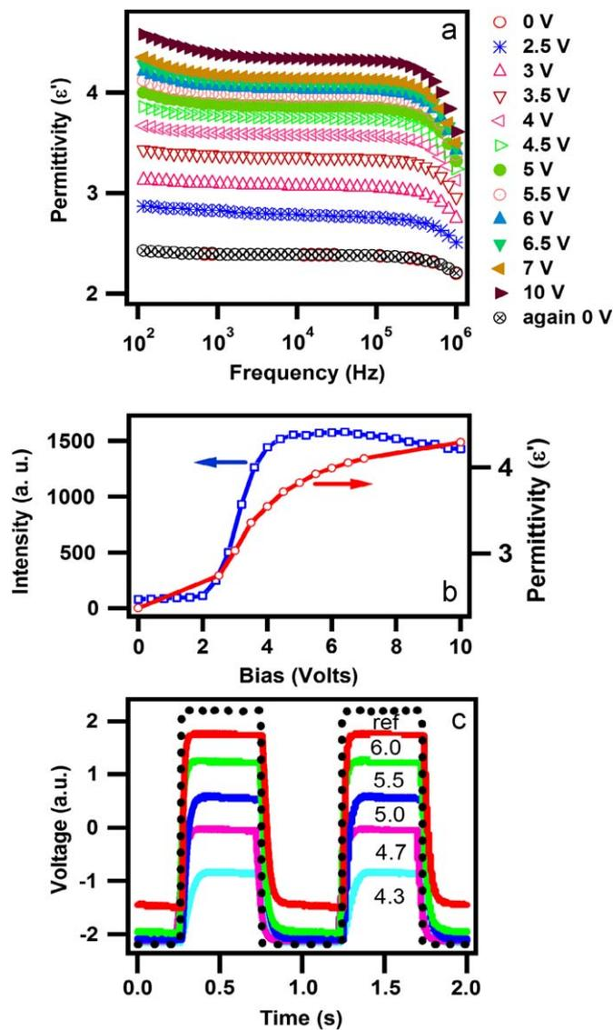
**Fig. 3.** (Colour online) At room temperature (a) frequency dependent dielectric permittivity ( $\epsilon'$ ) at different bias voltages, (b) dielectric permittivity ( $\epsilon'$ ) versus bias voltages at 20 KHz and steady-state (square wave 0–10 V @ 1 KHz) optical transmission at  $\lambda=633$  nm, and (c) time-resolved (ac bias 4.3–6.0 Vpp @ 1 Hz) optical transmission with white light.
