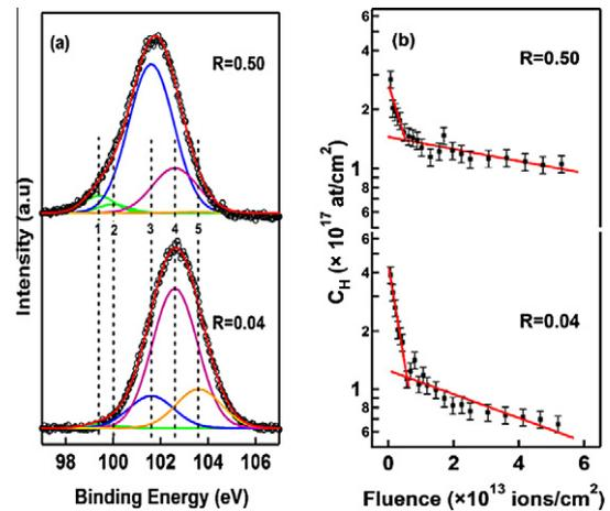
**Figure 2.** Representative XPS spectra for the as-deposited films corresponding to  $R = 0.04$  and  $0.50$ . (a) Deconvoluted Si  $2p$  XPS spectra: peaks 1 and 2 correspond to elemental Si, whereas peaks 3, 4 and 5 represent Si in  $\text{Si}_3\text{N}_4$ ,  $\text{SiO}_x\text{N}_y$  and  $\text{SiO}_2$  networks, respectively. (b) Variation of hydrogen concentration ( $C_{\text{H}}$ ) with fluence: solid lines (red) are linear fits.
