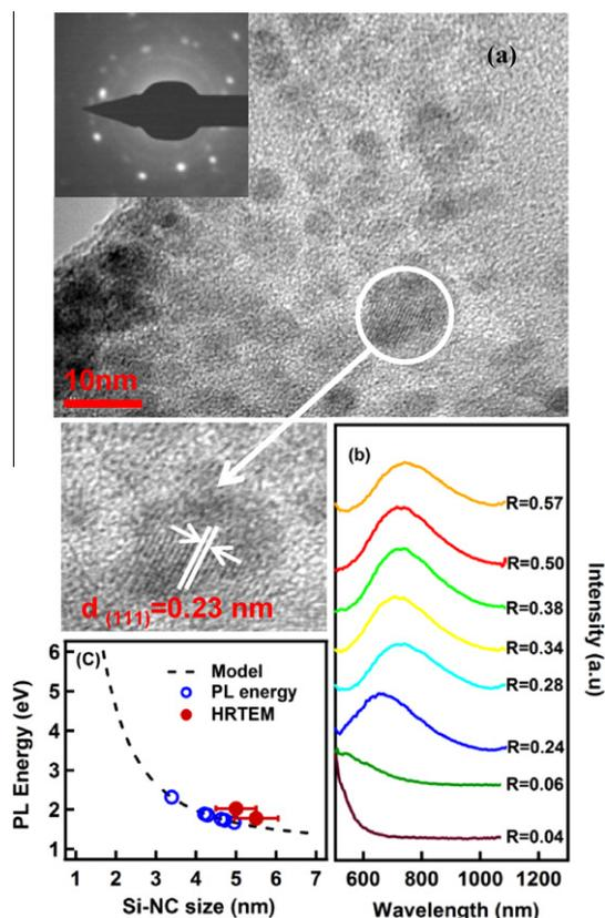
**Figure 3.** (a) HRTEM image along with SAED pattern for  $R = 0.50$  film. (b) Room-temperature PL spectra for different  $R$ -values. (c) A plot of PL energy vs. Si-NC size: open circles represent the estimated Si-NC size [17] from the experimentally observed PL peak energies and solid circles are PL energies corresponding Si-NC sizes, obtained from HRTEM data. Dotted line is model plot [17] as a guide to eye.
