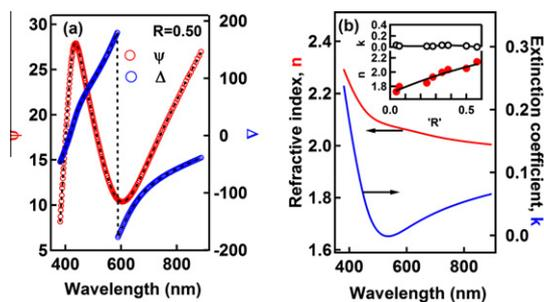
**Figure 1.** (a) Ellipsometer parameters  $\Psi$  and  $\Delta$  experimental and fitted values using a spline model for the film  $R = 0.50$ . (b) Optical constants: refractive index ( $n$ ) and extinction coefficients ( $k$ ) vs. wavelength plot obtained from ellipsometric analysis. Inset shows  $n$  and  $k$  (at 633 nm) values plotted as a function of  $R$ .
