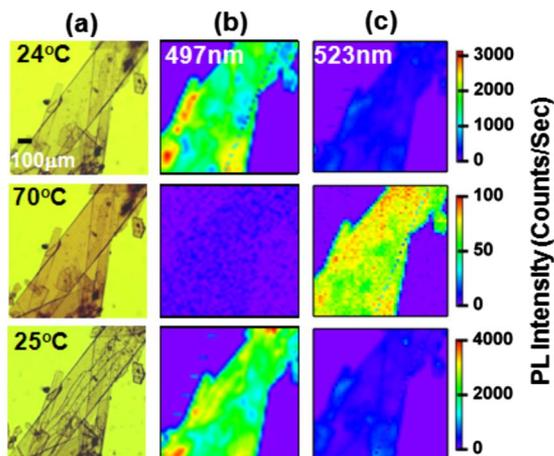
FIG. 3. (Color online) (a) Confocal transmission images of C12PI single crystals recorded at 24 °C, heated to 70 °C and cooled down to 25 °C. [(b) and (c)] PL images at each temperature for (b)  $\lambda=497$  nm phase-I and (c)  $\lambda=523$  nm phase-II excitons.
