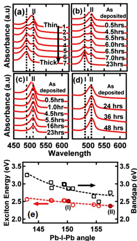
FIG. 2. (Color online) Exciton absorption of C12PI for effects of (a) film thickness and (b) aging (c) after annealing and (d) after PMMA capping of  $\sim 50$  nm thickness films. (e) plot of Exciton PL peak position and lowest bandgap vs Pb-I-Pb in-plane bond angle of various 2D hybrids (see text). Opaque circles are for PL maxima of C12PI phase-I and II. Dashed lines are guide to eye.
