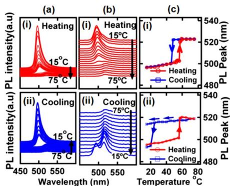
FIG. 4. (Color online) (a) C12PI crystal and (b) thin film (of thickness  $\sim 50$  nm) PL spectra during (i) heating and (ii) cooling between temperatures 15 to 75 °C and (c) Peak PL wavelength vs temperature on heating and cooling for (i) single crystal and (ii) thin film.
