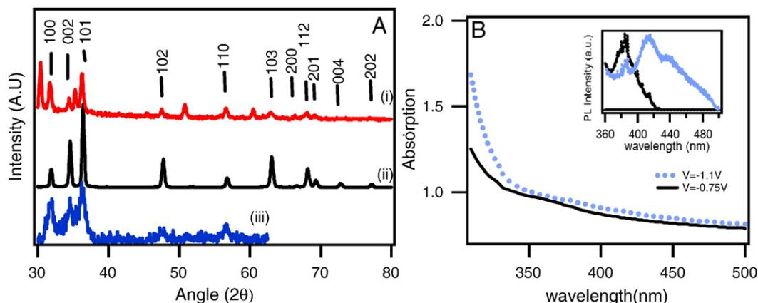
Fig. 2. (A) X-ray Diffraction of ZnO ((i) and (ii) are for electrodeposited thinfilm deposited at  $-0.75$  and  $-1.1$  V deposition potentials respectively and (iii) for synthesized nanoparticles; (B) Optical absorption spectra of electrodeposited thinfilm deposited at  $-0.75$  and  $-1.1$  V respectively. Inset is the photoluminescence of respective samples. (For interpretation of the references to colour in this figure legend, the reader is referred to the web version of this article.)
