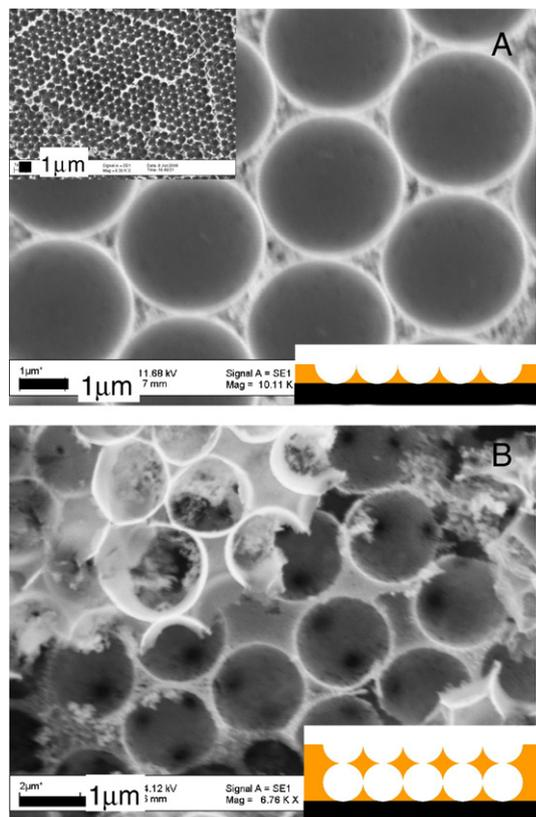
Fig. 3. SEM picture of microporous ZnO (inset of (A) is for  $700$  nm mesoporous ZnO). (A) and (B) are grown (as represented in the schematic figures) up to  $0.5d$  and  $>1.5d$  respectively, where  $d$  is the diameter of the templated spheres ( $d=3 \mu\text{m}$ ).
