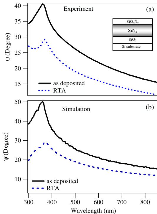
**Figure 2.** Ellipsometry analysis: (a) ellipsometer parameters  $\psi$  experimental and (b) simulations for as-deposited and RTA films. The inset shows a schematic representation of the three-layer model used in ellipsometry and XRR analysis (see text).
