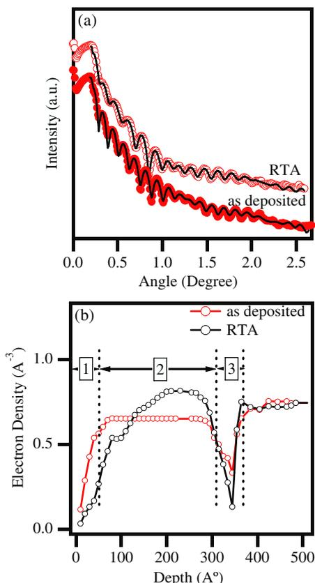
**Figure 4.** (a) GIXR spectra of as-deposited and RTA samples measured using  $\lambda = 1.5418 \text{ \AA}$  are shown along with fitted curves (continuous line). (b) The electron density profile obtained from the fit for as-deposited and RTA film. The three regions shown are described in the text.
