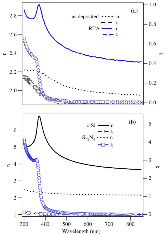
**Figure 3.** Plots of refractive index and extinction coefficients of (a) as-deposited and RTA films and (b) for c-Si and Si<sub>3</sub>N<sub>4</sub>, taken from [18].
